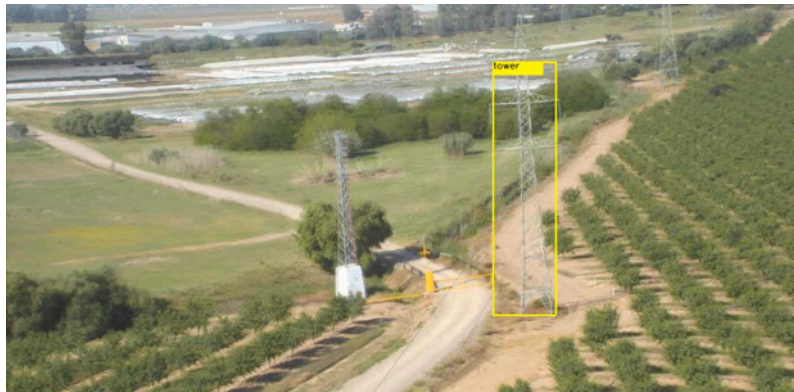
Figure 15. Sample output of the proposed 2D detection and tracking software.
