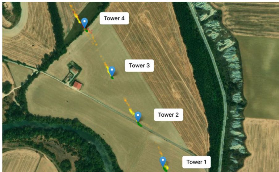
Figure 18. Object of interest actual coordinates and algorithm-generated coordinates comparison. Pins represent the real-world positions of 4 aerial cinematography targets. Red and orange dots are erroneous positional estimations that happen when the target is >120 meters away from the camera. Yellow and green dots are acceptable or accurate position estimations that are produced with targets 80 to 120 meters away from the camera.
