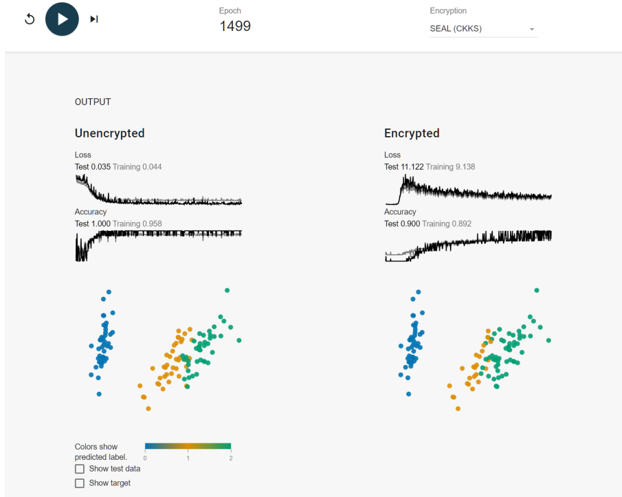
Figure 17. A screenshot of our demo application for encrypted inference. Complex FHE operations add noise to the data, which explains why the encrypted model converges slower than the unencrypted one
