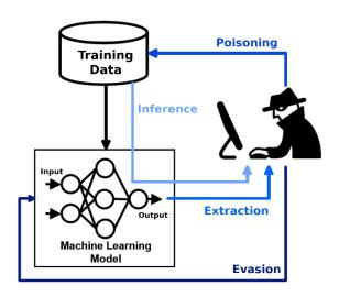
Figure 75: Different types of attacks against machine learning models. 327
