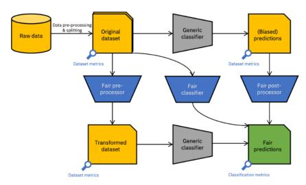
Figure 82: Various ways to mitigate bias in AI models. Bias should also be measured at multiple points in the AI lifecycle, including in deployment.
