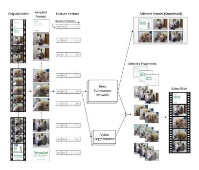
Figure 63: High-level representation of the analysis pipeline of deep-learning-based video summarisation methods for generating a video storyboard and a video skim.<sup>260</sup>
