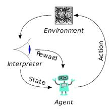
Figure 40: The components of the reinforcement learning framework.99
